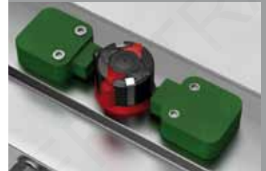
Mechanical switches indicating open and close
